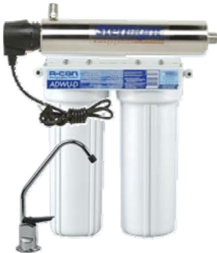
The **AWP ADWU-D** drinking water systems are designed for point-of-use water treatment. The **ADWU-D** is a double system with two white filter housings, which house a sediment removal cartridge and a taste, odors, chlorine and leads cartridge removal. The filter housings are NSF approved components, under standard 42.
